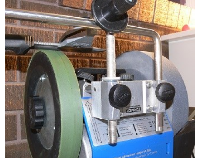
Match the ground angle with the honing angle
